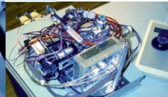
Mini-Positioner MT-55 driven by SMC-Corvus in a vacuum level of 10^{-3} mbar.
