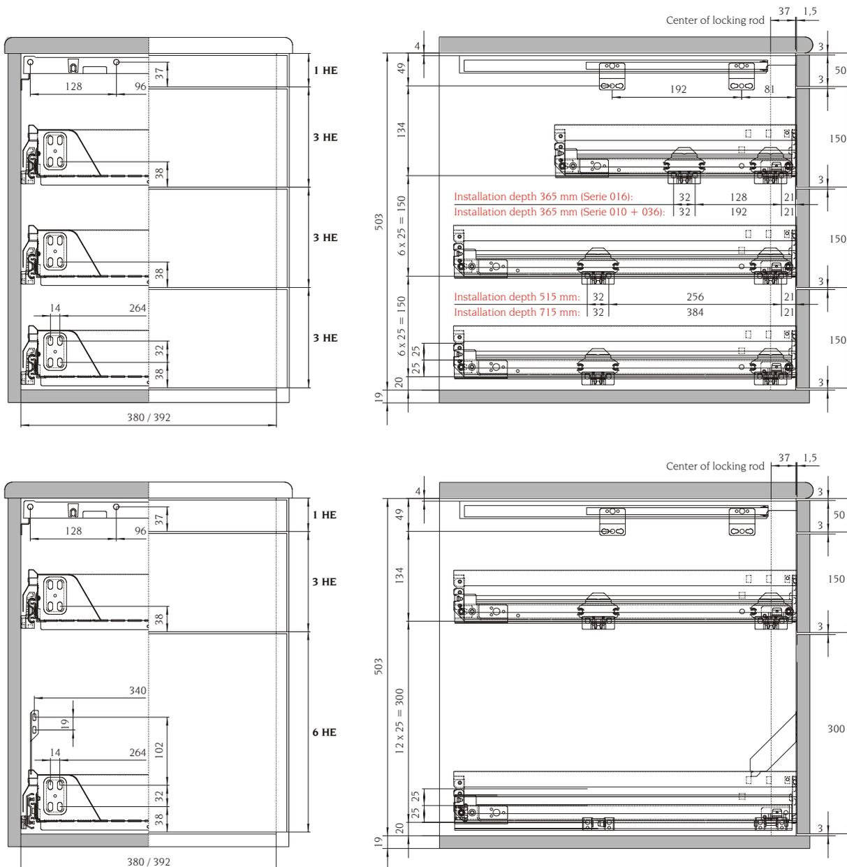
Drilling holes  $\varnothing$  5 for Euro screws (standard)
