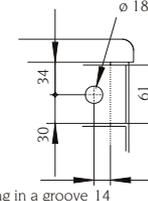
14 for locking rod running in a groove
