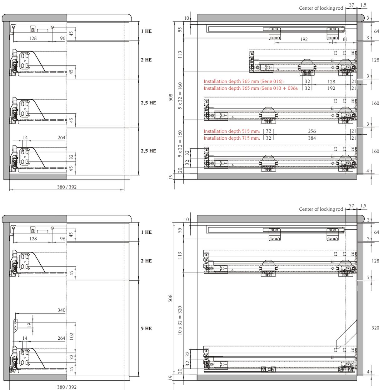
Drilling holes  $\varnothing$  5 for Euro screws (standard)
