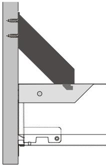
Insert the front panel supports in the upper slots on the drawer.
