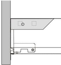
Insert the lock-catch plate (see page 10 for the complete selection) into the square holes on the front of the right shroud.
