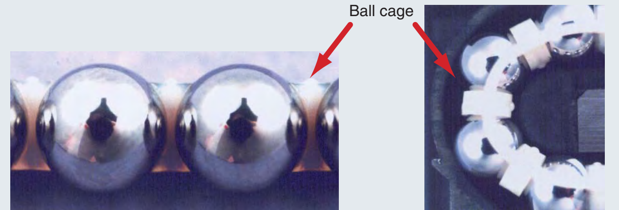
Contact state between balls and ball cage
