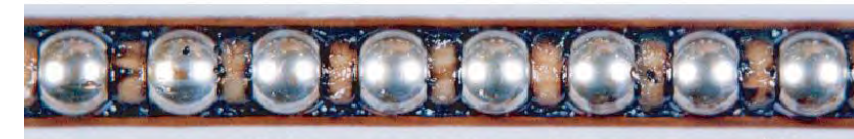
Ball cage after running 8,000 km Nominal life: L 10 = 400 km
