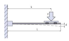
The deflection of a Slide beam acting as a cantilever and using a Long Flange Clamp (as shown opposite), will be a maximum at the free end when the load is at the outermost extremity of its stroke. This maximum deflection is given by the following equation:
