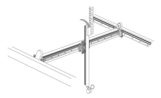
**SL2 System** is used as the means of guidance for all axes of a non-destructive ultrasonic testing machine. An ultrasonic probe is lowered into a spray tank during research in a university engineering department. For vertical guidance a special curved section stainless steel backplate manufactured by Hepco to the customer's drawing is incorporated, allowing an **SL2 Flat Slide** to be mounted to the circular section probe. The **SL2 System** is ideally suited to this humid environment.
