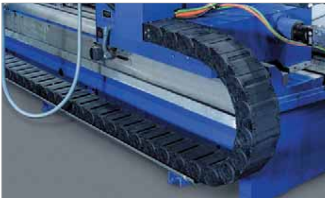
Type MT 0950 cable carrier on a roll grinding machine Installation variant: horizontal – "unsupported"
