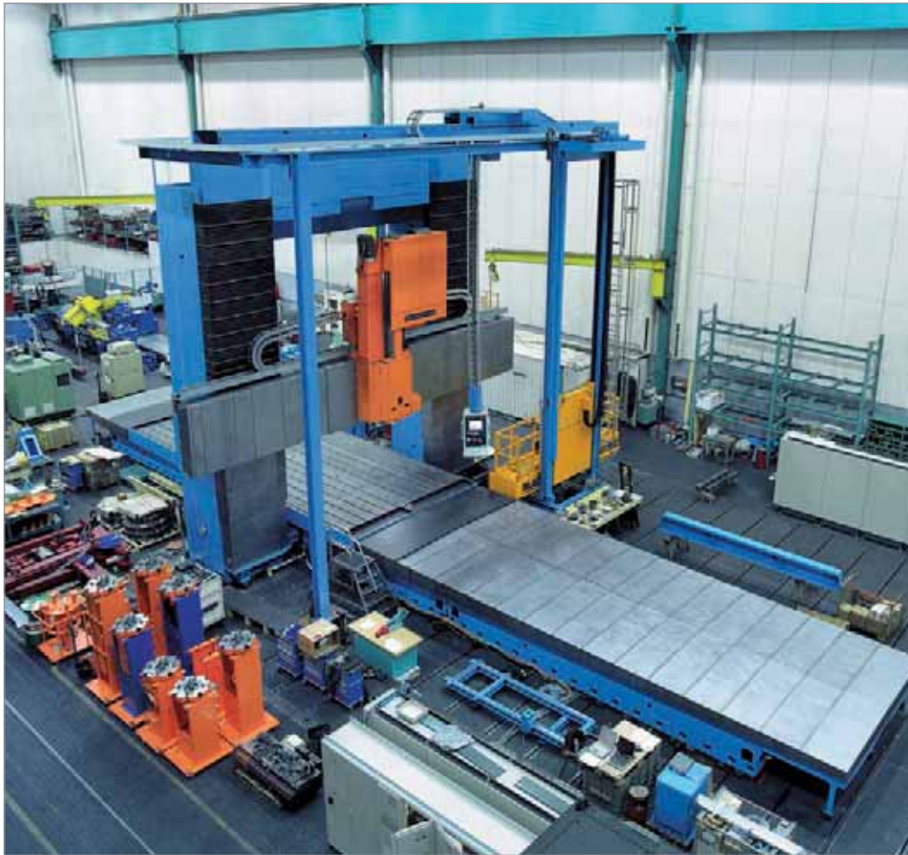
Steel and plastic cable carriers and KABELSCHLEPP telescopic covers on a portal milling machine
