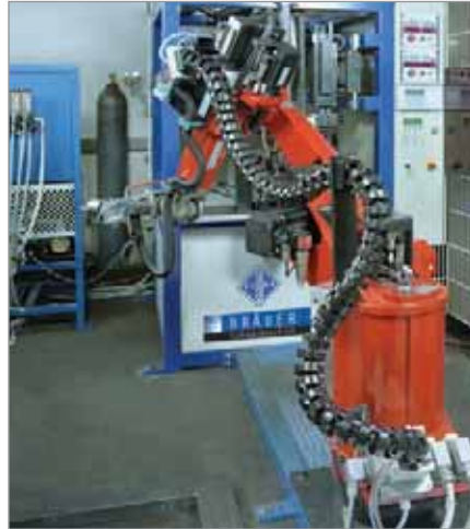
ROBOTRAX cable carrier system: Angle of rotation about 180° without channel system on a buckling arm robot application
