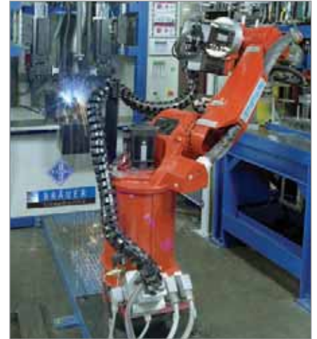
ROBOTRAX cable carrier system: Angle of rotation about 180° without channel system on a buckling arm robot application
