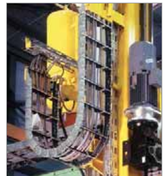
ROBOTRAX cable carrier system and steel cable carriers on a manipulator for handling crankcase core stackings
