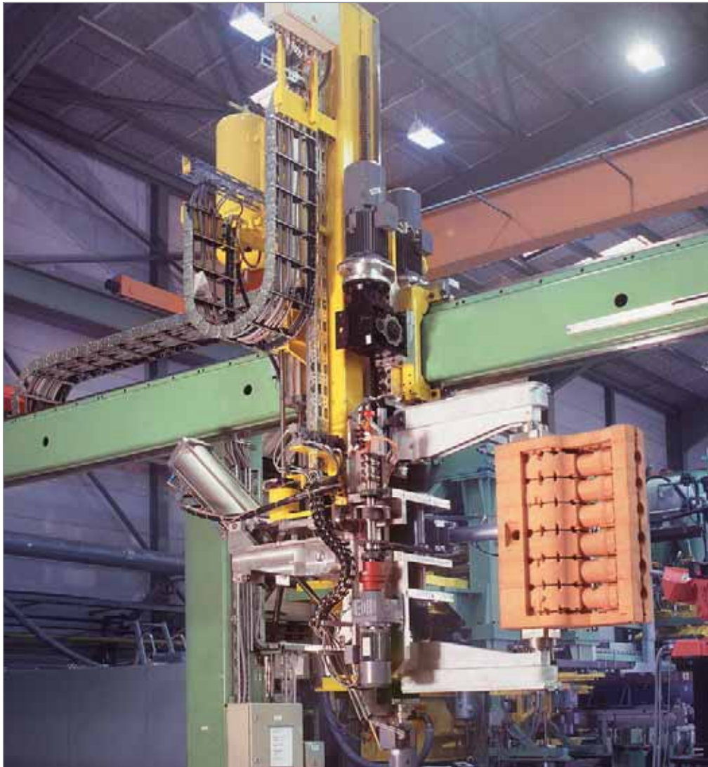
ROBOTRAX cable carrier system and steel cable carriers on a manipulator for handling crankcase core stackings
