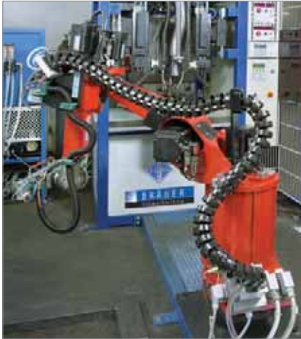
ROBOTRAX cable carrier system: Angle of rotation about 180° without channel system on a buckling arm robot application
