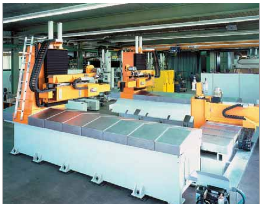
UNIFLEX Series cable carrier and KABELSCHLEPP telescopic cover on a highspeed machining center
