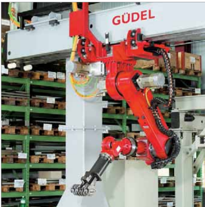
ROBOTRAX cable carrier system on a combined portal and buckling arm robot application
