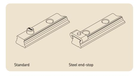
In addition to the plastic end-stop which is fastened in the first and last rail hole, there is also an option for a steel end-stop that can be mounted in any hole. Order suffix - M.
