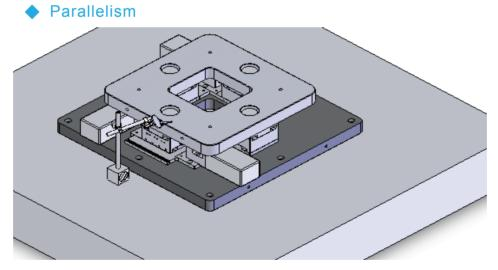
Put the alignment stage onto the bench under inspection; fully make measurements by sliding the test indicator. Now locate the bench at the stroke-middle point. Use the maximum deviation made during the bench-measuring zone as the measuring value.
