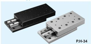
In the SVT type slide table, the slide way is sandwiched between an accurately machined steel tabletop and bed. In the SVTS type, an anti-corrosion SVS type slide way is sandwiched between an accurately machined aluminum tabletop and bed.
