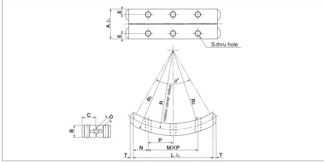
$\frak{\%}$  One set consists of 4 curved rails, 2 curved roller cages, and 8 end pieces.
