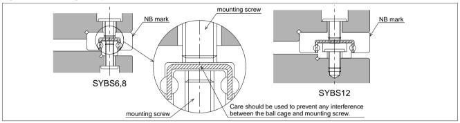
Table H-14 Mounting Screws (Material: Stainless Steel) Unit: mm
