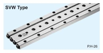
The SVW type slide way consists of two R type roller cages, two SV-type rails, and one W type rail with V-shaped grooves on both sides. The use of a W-type rail results in a compact design. The SVWS type is also available with all stainless steel components.
