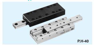
The SYT/SYTS type is a thin, compact slide table. Either tapped or counterbore type is available. The anti-corrosion SYTS type slide table is fabricated with all stainless steel components, making it suitable for use in clean rooms.
