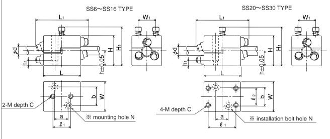
$\ensuremath{\overset{\scriptstyle <}{_{\scriptstyle \sim}}}$  The mounting holes are machined on request.
