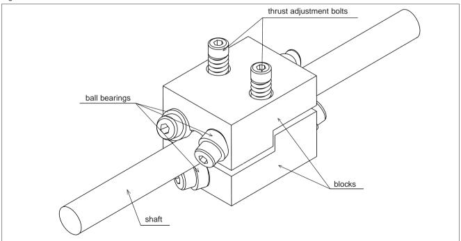
Figure J-1 Structure of NB Slide Screw
