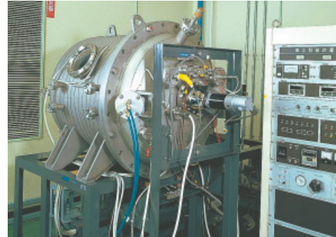
Photo 4.1 Vacuum testing system
