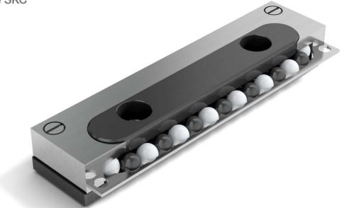
The recirculating unit type SKC was developed for dry running, vacuum and clean room applications. It is made out of DURALLOY® coated steel and has ceramic balls, which are separated from one another by balls made out of TEFLON®.
