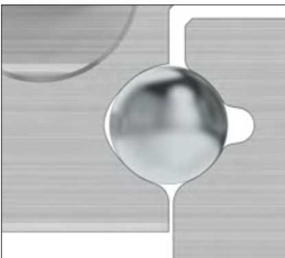
Gothic arc profile of the guideway tracks
