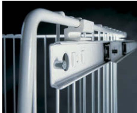
The fixing of this wire basket was developed especially for a North American manufacturer of refrigerators and deep freezers: Two plastic clips allow for tool-free mounting and easy removal of the basket by the end user.
