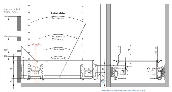
\* Regarding cabinets with a front cover, the hole pattern in the side walls has to be adjusted accordingly in case of additional tacks being used to stop the front cover 1-2 mm before the front edge of the cabinet.
