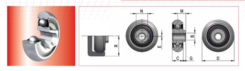
The rollers of series L.V and P.Z are single row bearings with 2Z steel seals.
