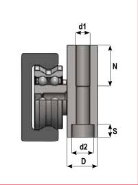
The A and B versions differ only in the arrangement of the rollers providing maximum radial load capacity either toward or against the mounting surface. The preferential loading direction is marked by two circular notches. (Ordering code example: RVT28-3A or RVT28-3B) The slider body allows two methods of mounting. One method is to pass a fastener through the counterbored hole into the payload or to pass a fastener through the payload into the tapped hole at M.
