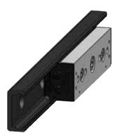
**RLV Series Sliders** RLV Series Sliders are made of strong Zinc plated steel body, with mounting holes parallel to the roller axles and perpendicular to the direction of preferred loading. The sliders have wipers with incorporate preciled felt for lubrication of raceways.
