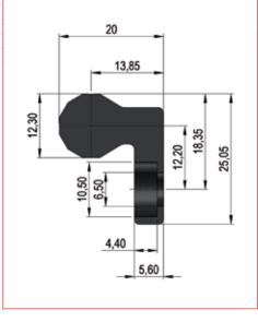
The rail is made from special carbon steel alloy to assure a good nitriding hardening with our T RACE-NOX treatment. An innovative hardening technology applied to the linear rail products able to increase the hardness on the surface and in depth, enough to guarantee to support the typical Hertz's stress in the point of contacts with the rollers, and to grant a strong resistant against corrosion, reducing the friction and the wear for a long life of the rail.
