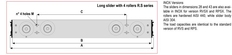
The extra long slider body for 4-roller sliders R.S..-4L are made to offer an economical alternative for the many cases where 2 sliders are used, merely for proportional reasoning, rather than for load capacities.
