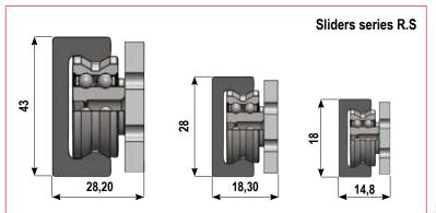
Sliders are available with either 3 or 5 rollers. For the 3 roller version, the first and third roller are fixed, concentric rollers that run on the same raceway. The second roller is eccentric and runs on the opposite raceway.
