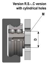
The sliders are available in standard version with threaded fixing holes R.S... and in version ...C with through passing holes for inside fixing with standard cylindrical screws DIN912, with no interference with the rollers.
