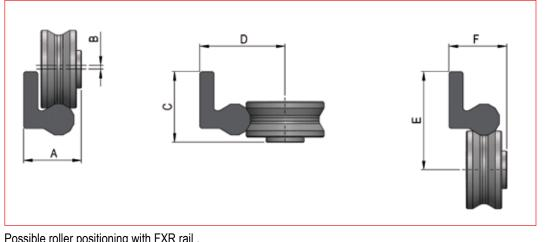
Possible roller positioning with FXR rail .
