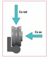
The roller must be correctly positioned with regards to load direction and too with sufficient number of rollers to assure requested load capacity and life-time.
